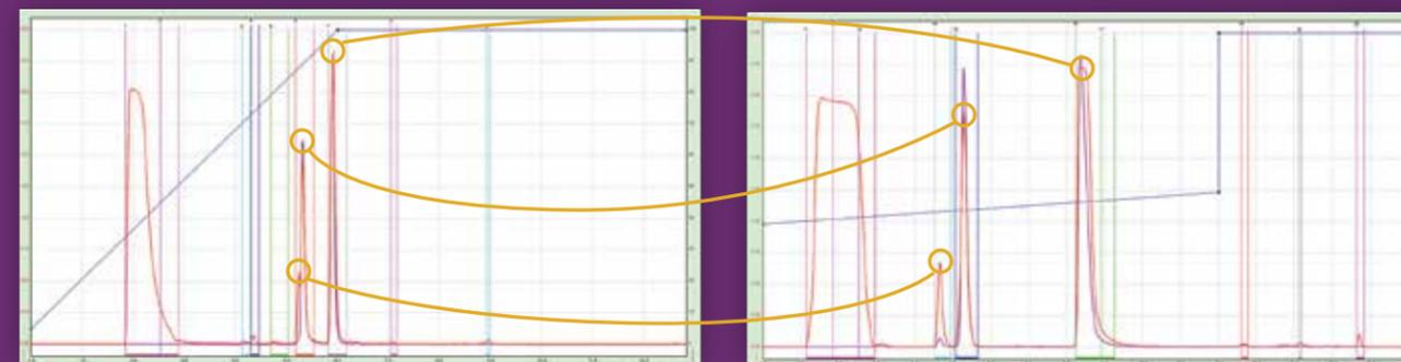
*Run a scouting run on the ACCQPrep SFC or from a calibrated analytical system and simply touch the peak of interest or enter its retention time for an optimized method for scale up.*
