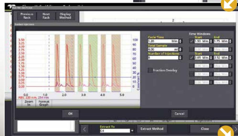
*The STACKED INJECTION WIZARD automatically suggests a cycle time, and time windows based on the isocratic run and simulates a series of stacked injections for the user to visualize. Simply enter your injection parameters and click OK.*
