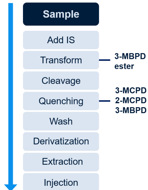
Figure 1: Schematic illustration of sample preparation according to the official AOCS Cd29a-13 method using the CHRONECT Workstation MCPD – Module ISO 18363-3.
